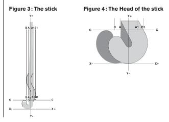
2.2 The shape and dimensions of the stick are tested by placing the stick playing side downwards on a flat surface marked with the lines shown in figures 3 and 4. Lines A, A1, B, B1 and Y are parallel and are perpendicular to lines C and X. The dimensions in figures 3 and 4 are:
